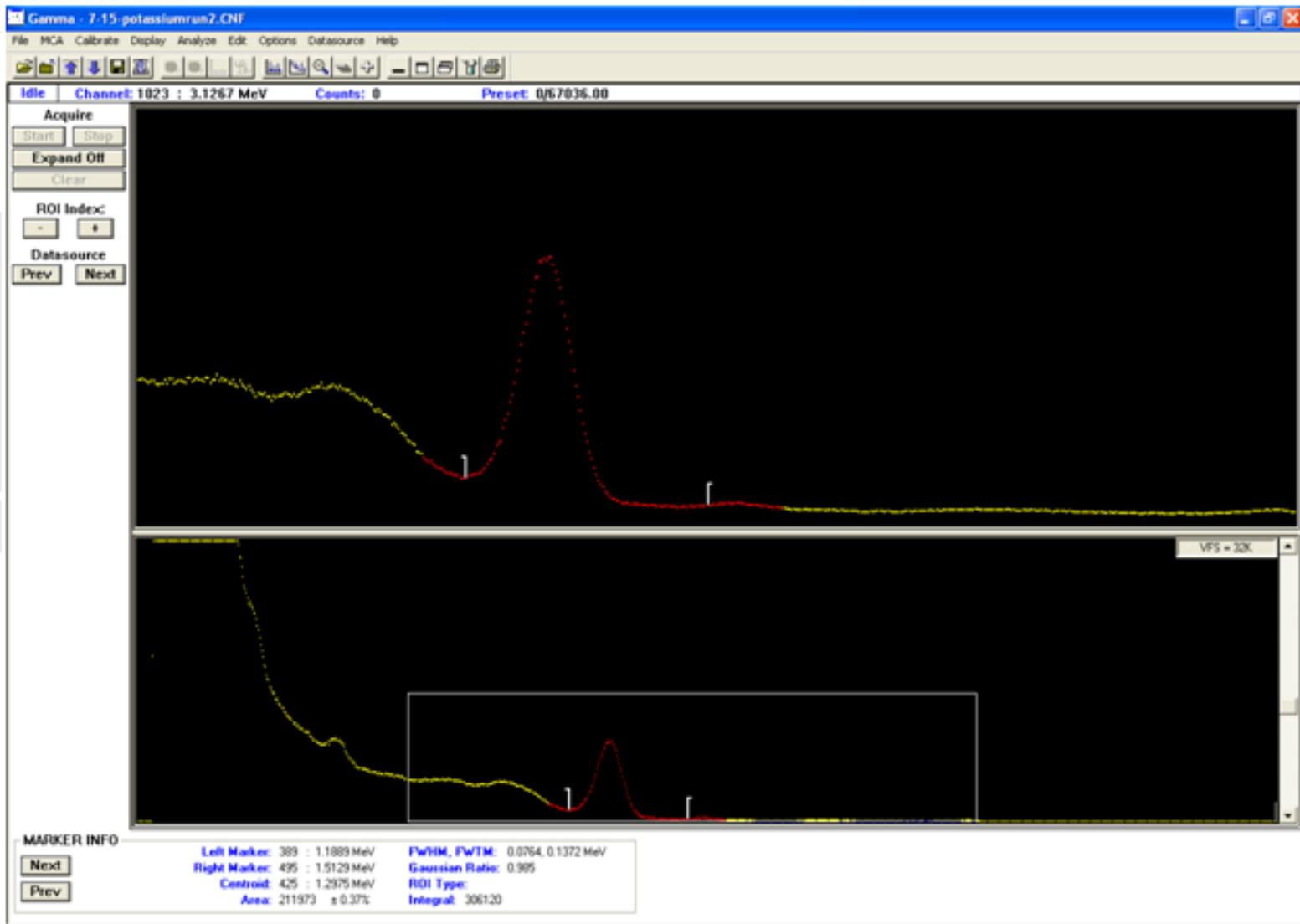
All data and count rates were analyzed in the region between 1.1889 MeV and 1.5129 MeV, which encompasses the peak of gamma radiation from K-40.
